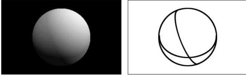
Figure 3: An example of the cut-off curves (right) corresponding to the image of a sphere (left) illuminated by two light sources. This type of image is analyzed in Zhang & Yang’s approach to recover multiple light sources.
